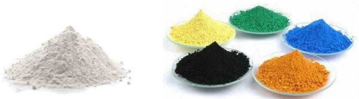
Titanium Dioxide, TiO_2 (left) and various mixed-metal oxide pigments used in the tinting of architectural coatings. These compounds have an extremely durable crystal lattice structure that resists the rigors of long-term weathering.
