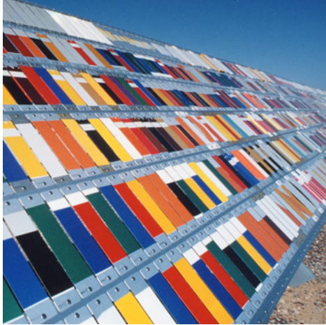
(Left) Test panels being evaluated at certified South Florida Laboratory. Note the 45-degree angle, Southward facing. (Right) A chart showing typical climate profile of South Florida. These conditions make it ideal for weathering exposure
